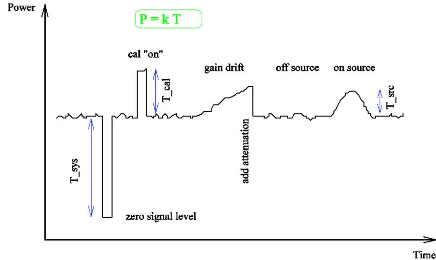
$$\frac{P_{off}}{P_{on} - P_{off}} = \frac{gT_{sys}}{g(T_{cal} - T_{sys}) - gT_{sys}} = \frac{T_{sys}}{T_{cal}}$$
