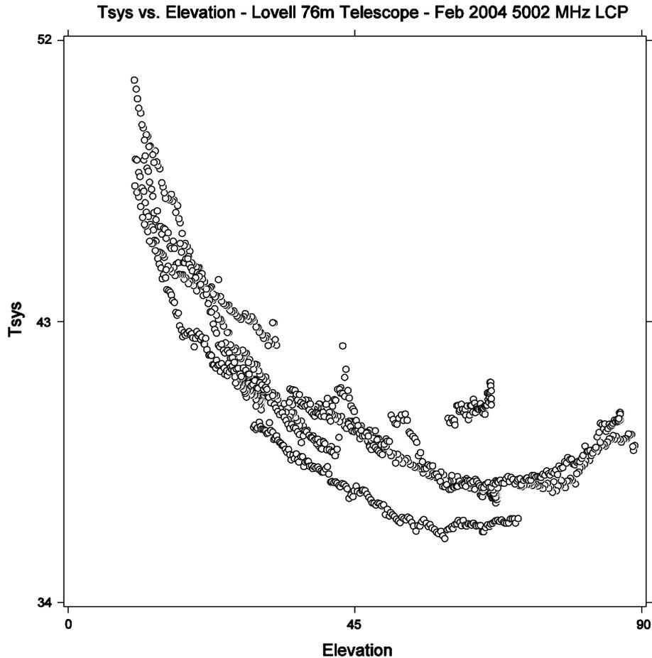
$$T_{\text{atm}} = T_{\text{zenith}} \left( 1 - e^{-\tau / \sin(El)} \right)$$
