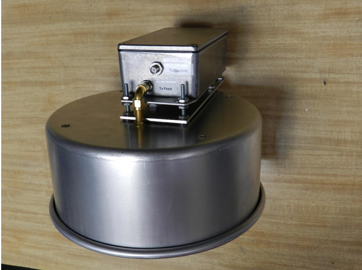
Figure 11: The completed feed and LNA assembly.
