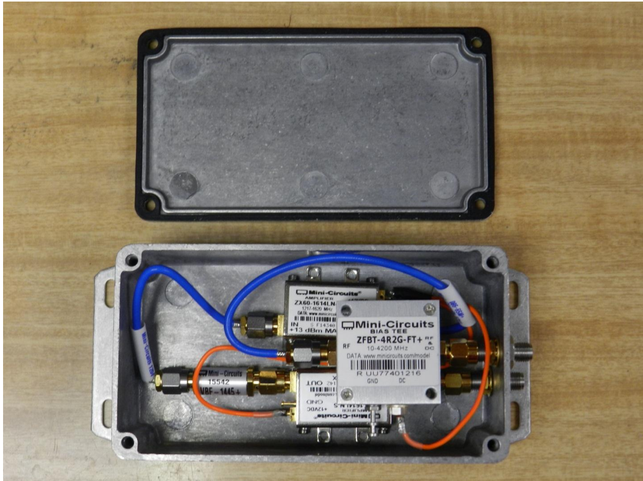
Figure 5: Completed LNA case with gasket on the lid.
