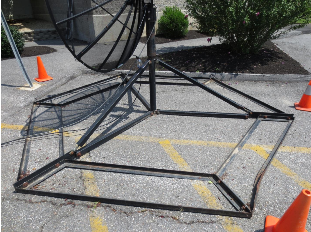
Figure 2: The Kaul-Tronics NPRM-10 mount for the prototype SRT. Concrete blocks or other counterweights should be placed in the six sections around the perimeter.
