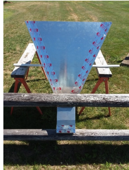
Figure 10: Back Profile antenna on stand
